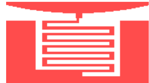
Type A Pure flexure, simple
