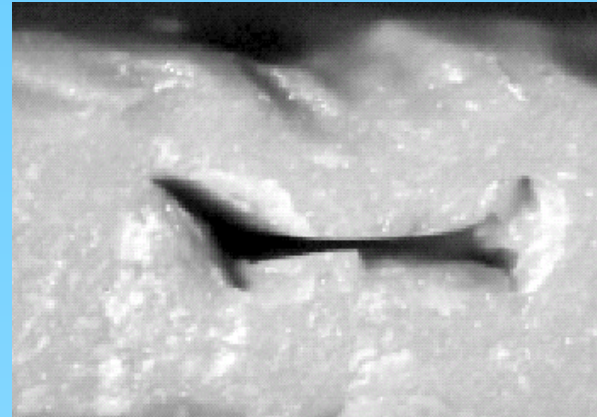
Cavity deformation after thermo-compression lamination
