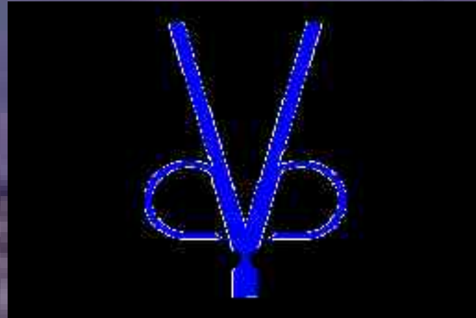
Feedback fluidic oscillator
