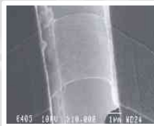
Figure 7: SEM picture of the hinge portion covered with a Ti/Au stripe
