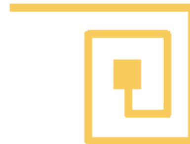
Example for designing an inductor on LTCC
