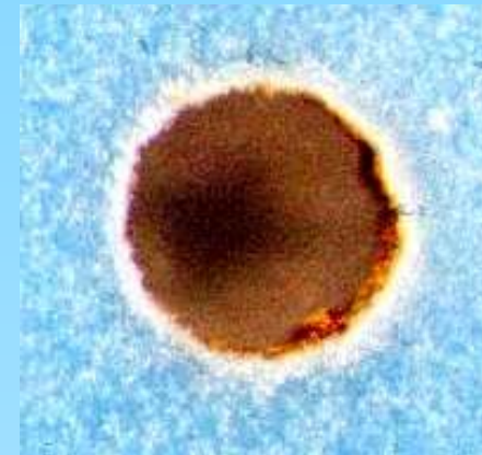
Nd-Yag Laser machined sample Excimer Laser machined sample Yag Laser Machined Via ( ~150 micron wide channel, 20X) (~ 40 micron holes, 20X)
