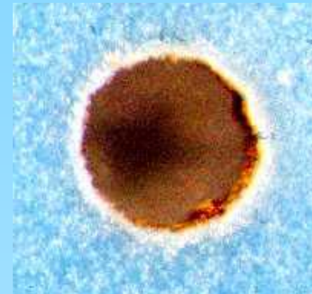
Nd-Yag Laser machined sample ( ~150 micron wide channel, 20X) Excimer Laser machined sample ( ~ 40 micron holes, 20X) Yag Laser Machined Via
